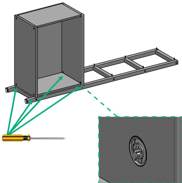
Using a screwdriver do up the cams on the Lower Storage unit. Slide the open storage on to the pins.
