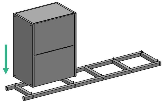
Slide Lower storage unit onto pins on the end frame.
