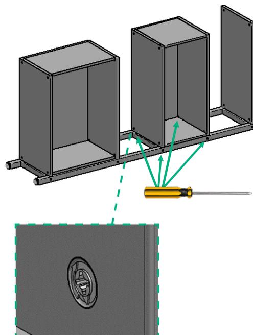
Do up the cams on the open shelf unit and install top shelf.
