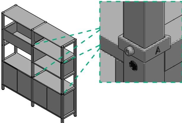
Attached clamp brackets to the Grid 40 frame.
