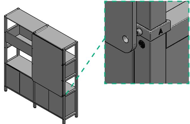
Push panel onto the clamp brackets.
