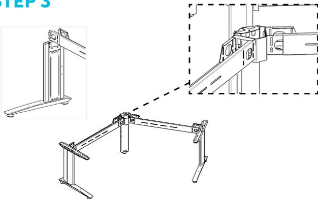
Attach the Extendable beam to the leg column as per above, the open side of the beam to the back. Use a nylon hammer to hit the top of the beam into place.
