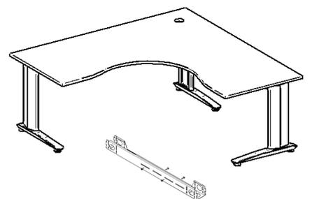
Using the bolts supplied with the beam, install 2 bolts front and back of each beam as per above.
