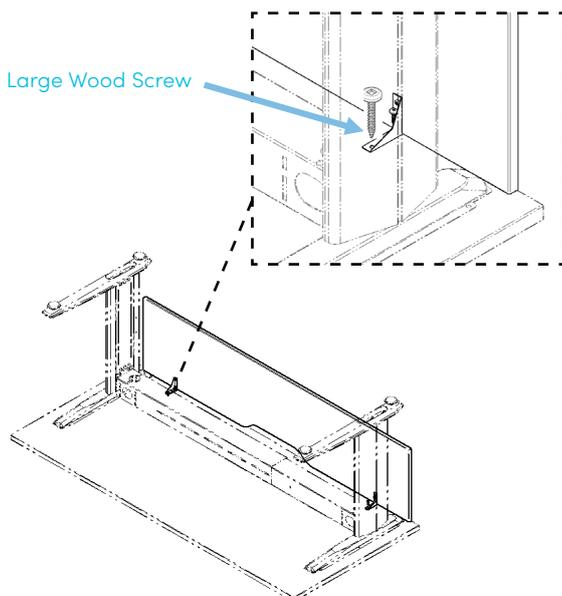
With the desk upside down attach the panel to back edge, using the large wood screws (10g x 19mm).
