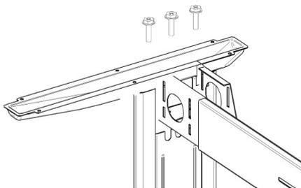
Attach Leg top plate to the top of the Leg columns using bolt A.
