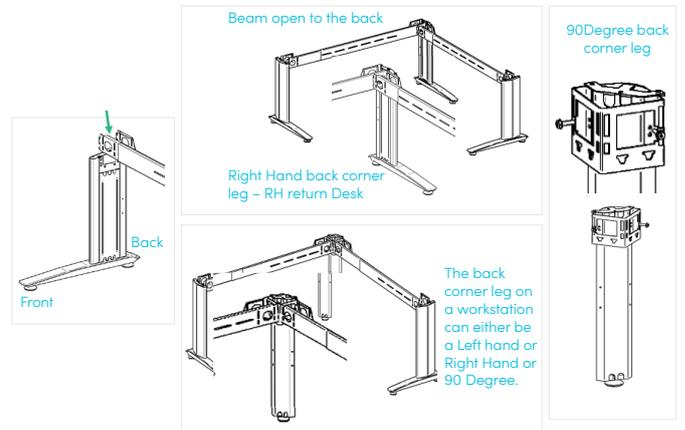
Attach the Extendable beam to the leg column as per above. *Note: The beam can be installed with the open side to either the front or back, depending on the preference of the user. Use a nylon hammer to hit the top of the beam into place.*
