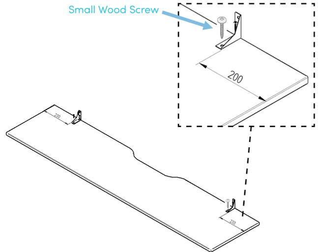
Attached the Brackets to the panel, using the Small Wood Screws (8g x 16mm).
