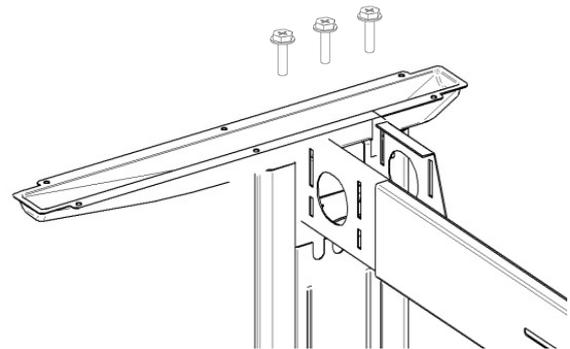
Attach the top plates to the leg columns using bolt A.
