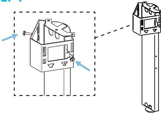
Attach 120degree bracket to the 120degree back corner leg as per above, using Bolts supplied with the bracket.
