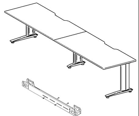
Using the bolts supplied with the beam, install 2 bolts front and back of each beam as per above.
