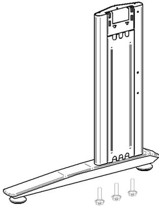
Attach Leg column to Foot, using bolt A. Make sure the bolt holes on the leg column are to the back of the foot as per above.
