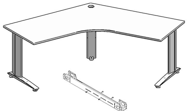
Using the bolts supplied with the beam, install 2 bolts front and back of each beam as per above.
