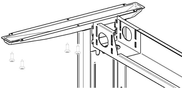
Place Desk top on the base frame, attach the desk top to the frame with bolt B.
