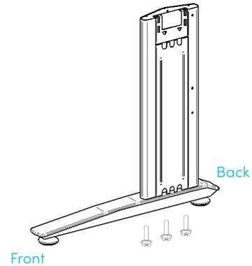
Attach Leg column to Foot, using bolt A. Make sure the bolt holes on the leg column are to the back of the foot as per above.
