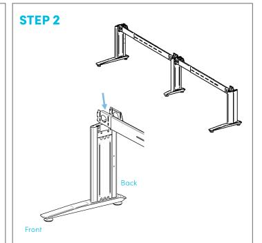
Attach the Extendable beam to the leg column as per above. Note: The beam can be installed with the open side to either the front or back, depending on the preference of the user. Use a nylon hammer to hit the top of the beam into place.
