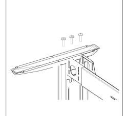
Attach Leg top plate to the top of the Leg columns using bolt A.
