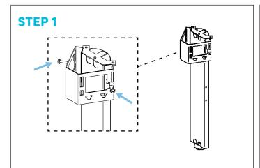
Attach 120degree bracket to the 120degree back corner leg as per above, using Bolts supplied with the bracket.
