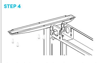
Place the desk top on the base frame, and extend the frame out so that holes on the top plate match the predrilled holes on the underside of the desk top. Attach the desk top to the frame with bolt B.
