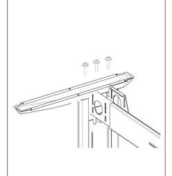
Attach Leg top plate to the top of the Leg columns using bolt A.
