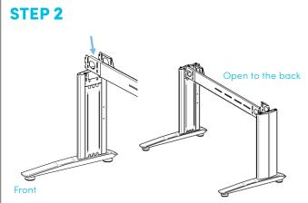
Attach the extendable beam to the leg column as per above, the open side of the beam should face the back.
