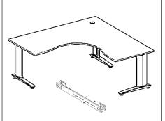
Using the bolts supplied with the beam, install 2 bolts front and back of each beam as per above.
