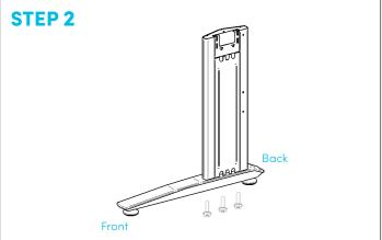
Attach Leg column to Foot, using bolt A. Make sure the bolt holes on the leg column are to the back of the foot as per above.
