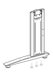
Attach Leg column to Foot, using bolt A. Make sure the bolt holes on the leg column are to the back of the foot as per above.
