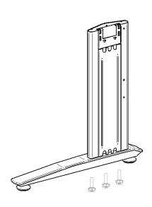
Attach Leg column to Foot, using bolt A. Make sure the bolt holes on the leg column are to the back of the foot as per above.
