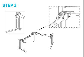
Attach the Extendable beam to the leg column as per above, the open side of the beam to the back. Use a nylon hammer to hit the top of the beam into place.
