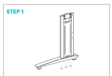
Attach Leg column to Foot, using bolt A. Make sure the bolt holes on the leg column are to the back of the foot as per above.
