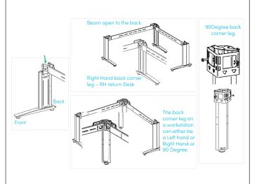
Attach the Extendable beam to the leg column as per above. Note: The beam can be installed with the open side to either the front or back, depending on the preference of the user. Use a nylon hammer to hit the top of the beam into place.
