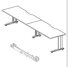
Using the bolts supplied with the beam, install 2 bolts front and back of each beam as per above.
