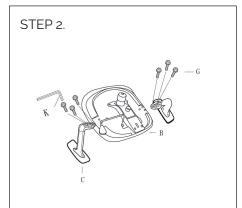
Please be careful to use the correct Arm Screws (G), For easy assembly, place the Seat (B) face down on a flat surface. Attach Armrest (C) to the seat (B) as shown using 3 Arm Screw (G) on each arm. Tighten the bolts securely with the enclosed Allen Wrench (K).
