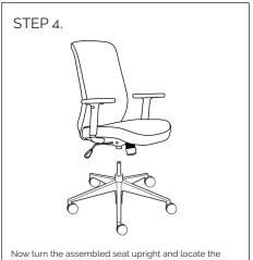
Now turn the assembled seat upright and locate the centre hold of the Mechnism over the Gaslift.
