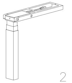
2. Install Upper Side Support with Screw. (Pic3 and Pic4) (Parts: 2pcs M6x16).
